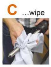
The solid stainless steel sensor is simply immersed into the fluid to obtain an immediate viscosity measurement. There is no limit on vessel size or fluid volume, so long as the tip of the probe is covered. Simply wipe clean after use.
